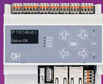
LON-Router = DHCON + Routing Software
