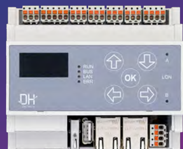
DHCON = DHCOM + Carrier Board + Housing
